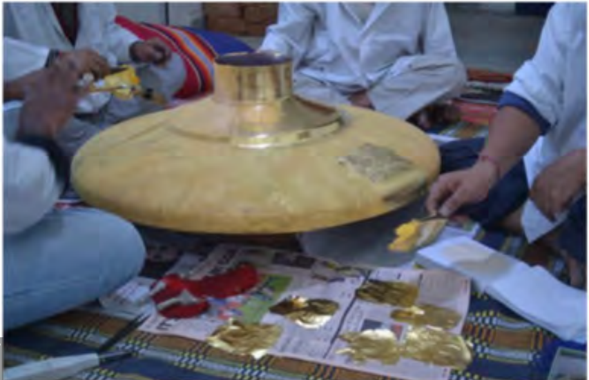
After the application of gold foils, each vessel was polished using glass beads and given the final finish
