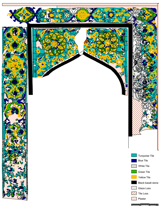
Architectural documentation of the tile work on the southern facade of the Ibrahim Quli Qutb Shah's Mausoleum
