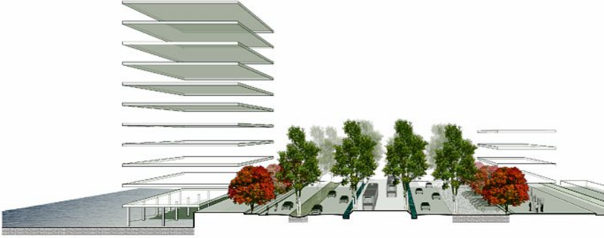
Civic Spine south (urban area): in the southern part of O Mon, with a symmetrical configuration and public transportation in the center
